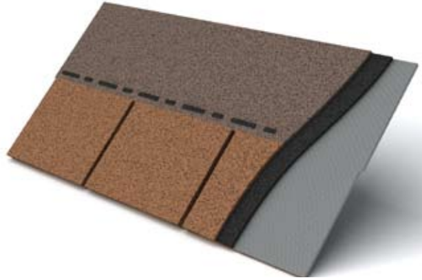
Three layers of an asphalt shingle
