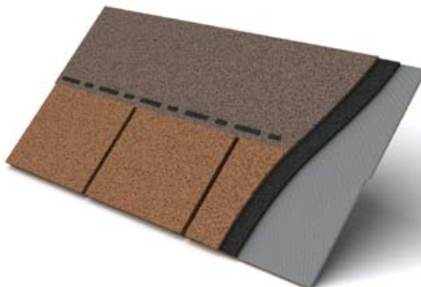
Three layers of an asphalt shingle
